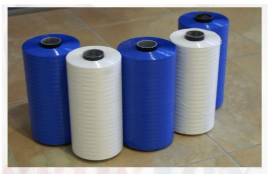
These yarns are high modulus PP which is obtained by increasing the draw ratio of material The application of these yarns can be for the backing of woven carpets. Count - dtex 890 - dtex 1440 Fibrillated - yes Colour-possible upon request
